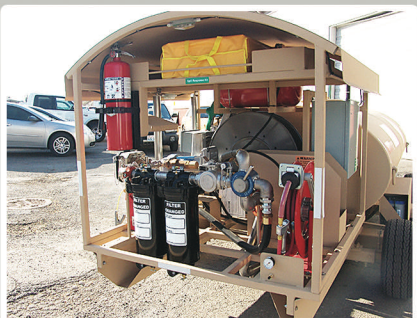
Back view shows dual stage filters, fire extinguisher, spill kit, and defuel/fuel select valve
