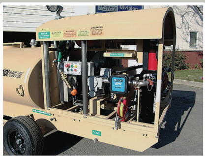
Operator's position - Note the simple control panel, meter, grounding reel and hose guides
