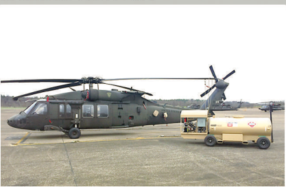
Side view of unit - note the mobility friendly fork-lift pockets and heavy-duty tie down points
