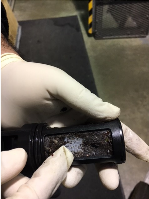
Figure 4-16 Clogged Pump Strainer
