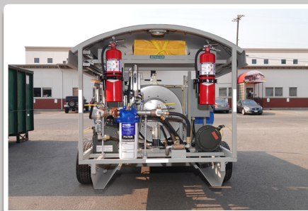
This is the rear view. Here are the fire extinguishers, the spill kit, the filter housing, as well as the fuel/defuel valve and pre/post filter fuel sample ports.
