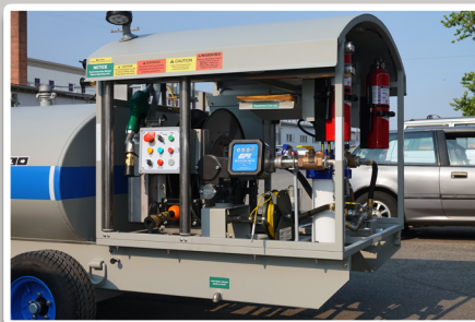
Operator's panel with access to controls, meter fuel log storage, grounding reel, and fuel nozzle. Notice the two vertical stainless steel hose guides.
