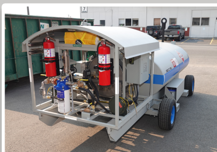
Right side where we find the weatherproof electrical box that houses the charger. Also here is the storage area for the optional SPR nozzle. Note the NATO plug on the electrical box.
