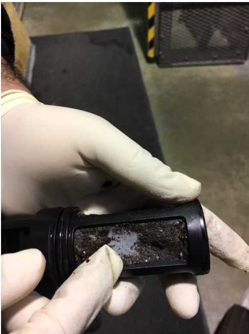
Figure 4-16 Clogged Pump Strainer
