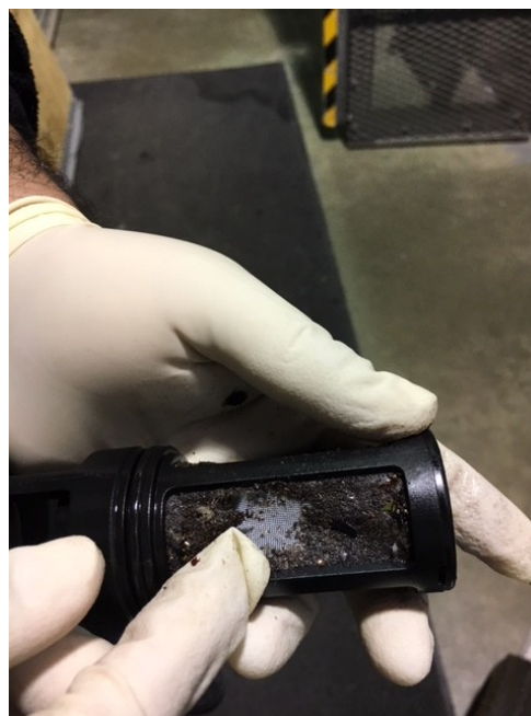
Figure 4-15. Clogged Pump Strainer
