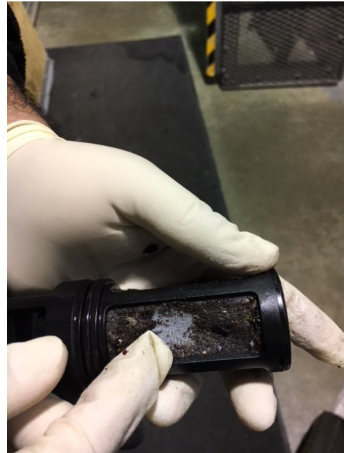
Figure 4-15. Clogged Pump Strainer
