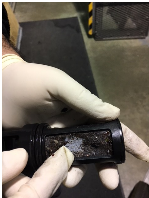
Figure 4-16 Clogged Pump Strainer
